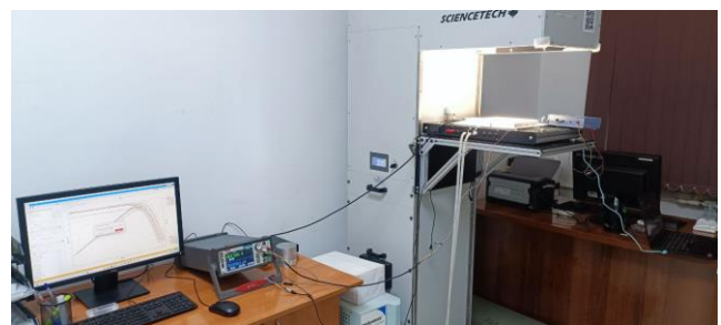
Fig. 3. Measuring VAC of modules using the Sciencetech solar radiation simulator (UHE-NL-250)
