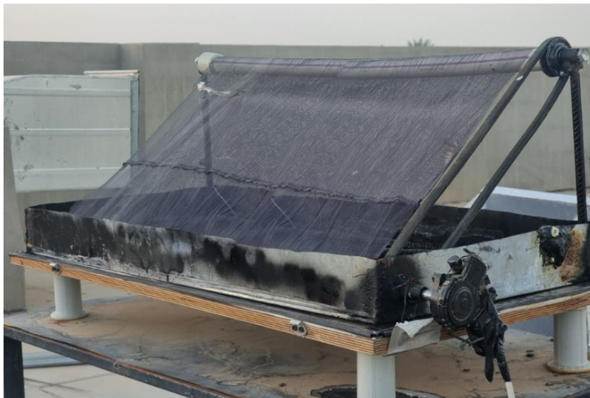
Fig. 3. Cotton mesh connected to a 12V motor inside the improved solar still
