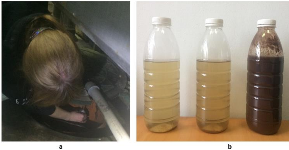
Fig. 3. General view of the sampling site of wastewater after the settling tank (a) and recirculation water after the mechanical filter, wastewater and sludge after settling in the settling tank for a day (b)
