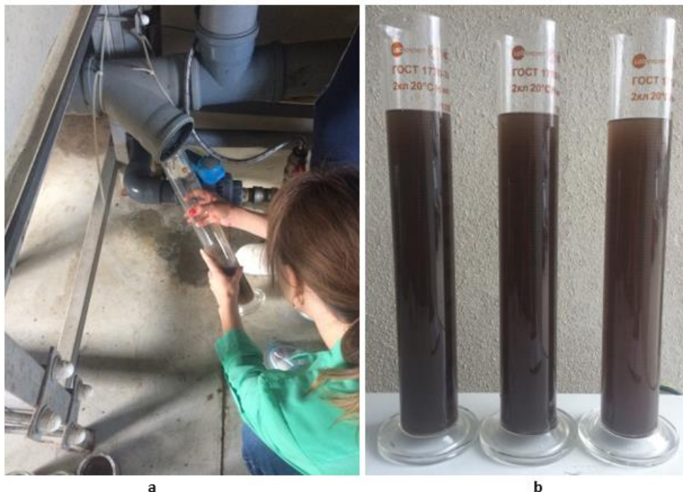
Fig. 2. General view of the sampling site for the waste wash water (a) and the wash water from the mechanical filter in the measuring cylinders (b)
